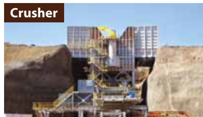
Crusher • Number: 4 • Size: 21m in height x 16m in width x 18m in length • Weight: 1,500 tonnes per unit • Capacity: 4,250 tonnes per hour per unit
