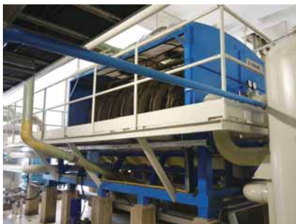
Desulphurisation gypsum and dehydration GDYT filter for power plants developed by CITIC Heavy Industries
