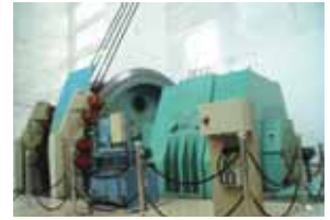
Large size hoist (Coal mining)
