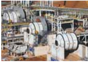
Large size grinding mill (Mining industry)
