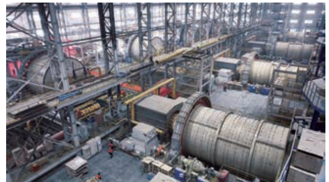
Mining capital equipment such as ball mills and semi-autogenous mills
