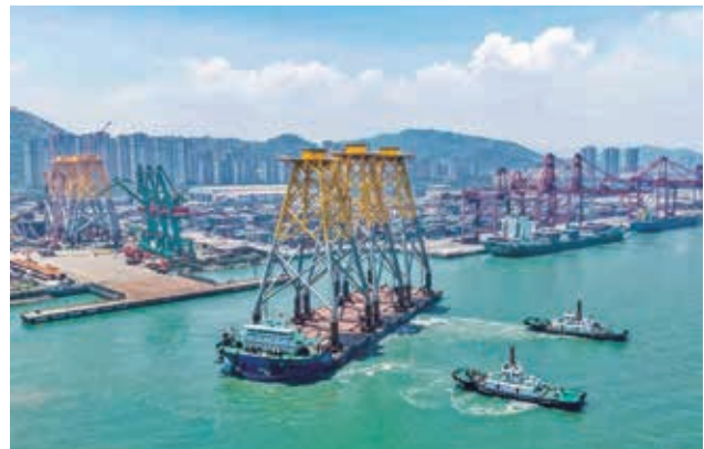
The offshore wind power jacket was shipped
