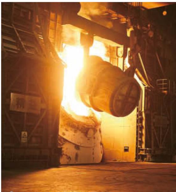
Converter process for steelmaking
