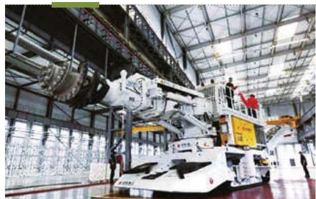
■ China's first T3.20 cantilever roadheader
