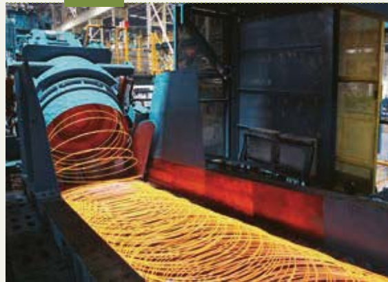
The production line of CITIC Pacific Special Steel's 2000 MPa grade cable wire coils
